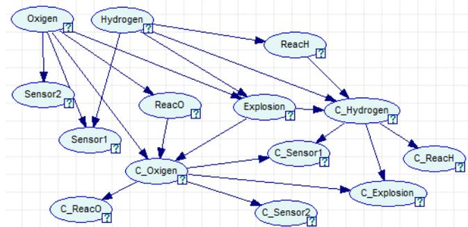
Figure 4: Bayesian Net screenshot from GeNIe (Decision Software Laboratory at <http://genie.sis.pitt.edu>) depicting the probability of an explosion and the ability of sensors to detect relevant factors.
