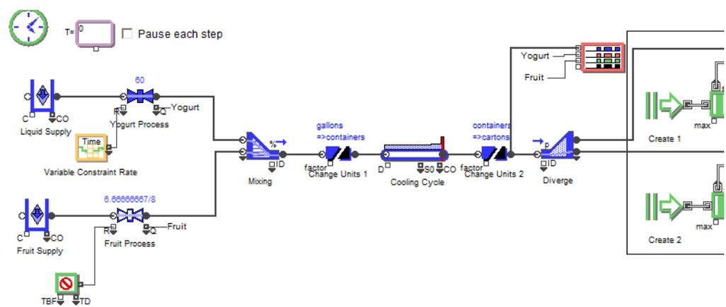
Figure 8: Screenshot of section of ExtendSim demonstration model of a yoghurt manufacturing process (ExtendSim model copyright © 1987-2010 Imagine That Inc. All rights reserved).
